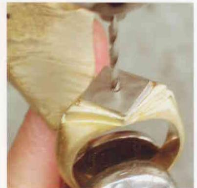
Enlarge the diameter of the pilot hole using a lubricated reamer bur. Constantly check while burring to make sure your enlarged hole is centered in the plate. Again, use moderate speed with constant torque.
