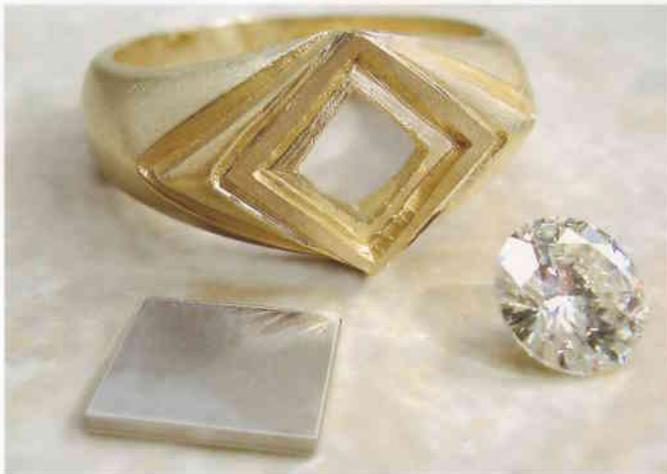
This 14k yellow gold men's ring casting will be prefinished, the platinum top soldered and the ring finished. The final step will be bead and bright cut setting of a 7.5mm stone.
