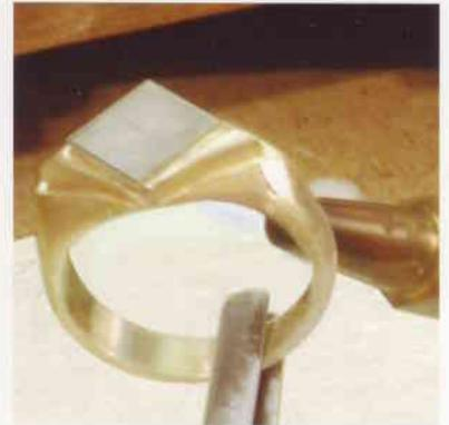
With the ring secured in a ring clamp, drill a pilot hole in the top using the number 30 handpiece and lubricated standard twist drill. With platinum, a moderate speed with constant torque is required.
