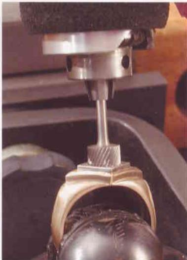
Place the gemstone in its bearing. The top of its table should be even with or slightly higher than the surface of the platinum top. All that's left is the bead and bright graver work.
