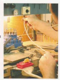
Dickey uses a tungsten carbide bur and the Foredom micromotor to remove the most interesting and colorful section of the shell. From this, he fashions a smaller piece suitable for the pendant. (He wears a face mask when working with the abalone to avoid breathing in the dust generated from the process.)
