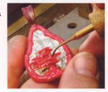
Because he took care to cover the shell with a wax lubricant, he's able to easily lift off the wax design to prepare it for casting.
