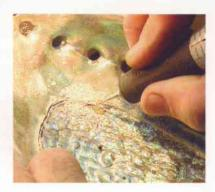
The shell is covered with a lubricant so the wax won't adhere to it during the build-up process. Dickey mounts the Foredom WC-1 Wax Carver temperature control box to the upright shelf above his bench. The on/off switch also controls the amount of heat to the tip. He turns on the unit and sets it to the desired temperature. The tip quickly reaches and holds the temperature.
