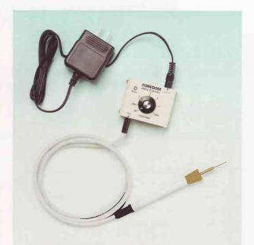
The Foredom Wax Carver WC-1control box measures 21/2" by 2". The transformer plugs into the top portion of the unit and an electrical outlet. There is a "power on" indicator light on the top left corner that flashes constantly when the unit is on. Approximate tip temperatures range from: Low—95°, 2—200°, 3—340°, 4—425°, 5—525° and Max is about 560°. A 230 Volt model with transformer adapters for European and British electrical outlets (WC-2) is also available from Foredom.
