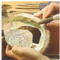
Dickey keeps a large reservoir of unmelted wax above his bench pen. With the supplied small spoon tip, melts and transfers the wax to the rim of the pendant. The handpiece is lightweight and the flexible cord can be detached from the power supply. The cork keeps heat away from Dickey's hands.
