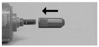
3. Screw sheath connector onto motor.
