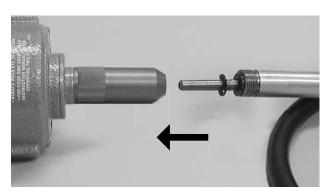
4. Lightly grease tip of shaft. Align the slot in tip of shaft with pin and slide into connector. Connect flexible shaft to motor shaft by aligning the slot in the flexible shaft onto the pin of the motor shaft adapter. Finally screw outer sheath into motor connector.
