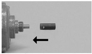
2. Place shaft adapter on motor, even with hub. Tighten setscrew.
