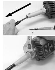
**5. Loosen set screw on the flexible shaft motor coupling and slide shaft off the motor shaft.**
