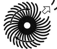
**Be sure you check** direction of brush/disc rotation. Running in the wrong direction can cause bristles to break off.
