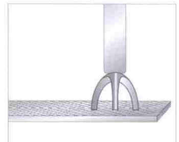
Make sure each prong is at the same angle and the same length. File the top of the prongs flat.
