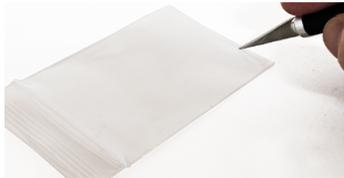
5. Carefully make a hole in the bottom of the 3" x 2" bag provided that is just large enough to slide in the shank end of the bur.
