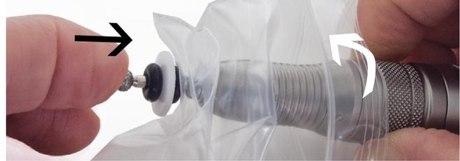
7. Tighten the collet with the bur inserted in as far as possible. Depending on your handpiece, you may need to push the bag forward on the handpiece in order to turn the knurled ring that tightens the collet.
