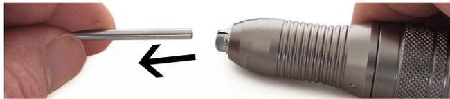
4. Remove test bur from handpiece and keep collet in open position.
