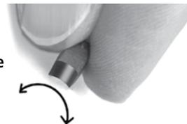
3. Re-insert brush assembly or new brush assembly into brush tube. Replace and tighten screws.
