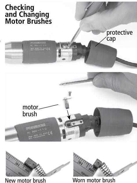
**When you reinsert a motor brush the curve should align with the handpiece contour**
