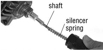
Slide both the outer sheath and the silencer spring off of the flexible shaft. Usually the silencer spring remains inside the sheath when you remove it.
