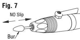
**Procedure** above and re-adjust the collet until the bur cannot be removed with the collet closed.
