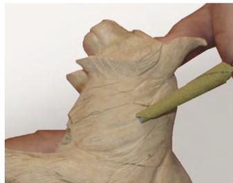
5. The long narrow point of the pattern should end up on or near the base of the roll on the mandrel body. If it doesn't, unwrap the abrasive and cock the edge in the slot (forward or backwards) slightly to bring the point back to the base of the roll on the mandrel once it is re-rolled.
