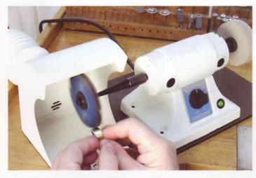
This bench jeweler has several rounded wide 14k yellow gold bands to prefinish. Here he's using a 3M Radial Bristle Disc. Prior to this step, he used the 3M XK Wheel to remove the sprue. The Foredom Lathe is mounted on a small board so it can be moved from one bench to other shop locations for various needs.
