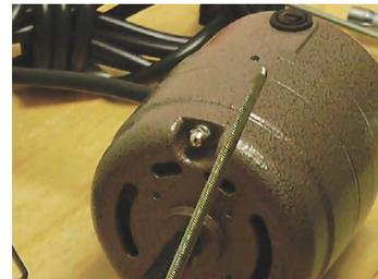
**5. Remove the motor brush caps and then the motor brushes from the motor housing.**
