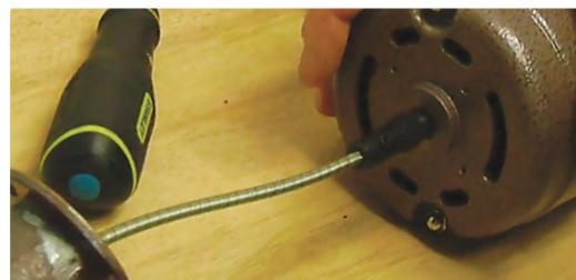
**4. Loosen set screw on drive link extension with 5/64" hex key.**
