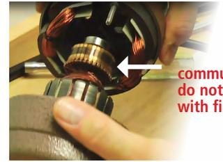
10. Reinstall the 2 motor brushes. Align the curvature of brush with the curvature of the motor.
