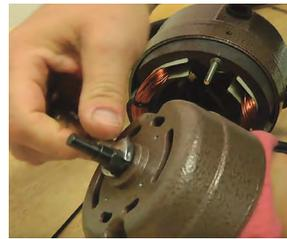
9. Wipe the commutator with clean cloth and reassemble the housing with the 2 acorn nuts. (Do not touch commutator with bare fingers.)
