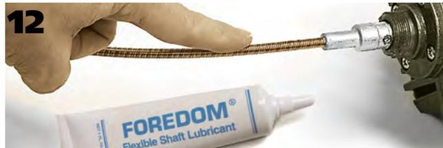
13. Bronze silencer spring should be inside the sheath assembly. Thread the new shaft into the motor hub and through the outer sheath assembly.
