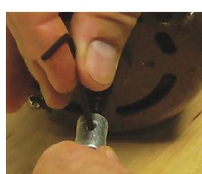
12. Apply a light film of Foredom grease MS10006 to flexible shaft assembly stopping 1-ft. short of the handpiece end.
