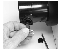
Remove motor brush
