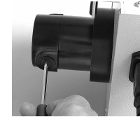
Unscrew brush caps on back of unit
