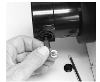
Remove motor brush
