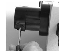
Unscrew brush caps on back of unit
