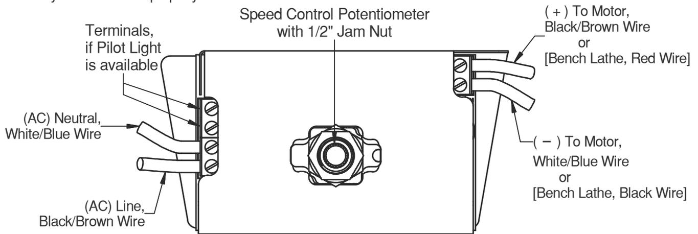
Top View of Circuit Board Assembly
