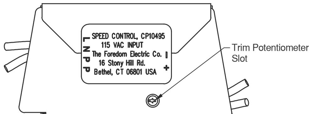
Bottom view of Circuit Board Assembly
